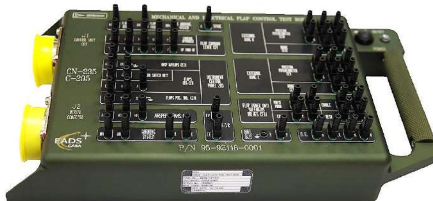
Fig. 3 Mechanical & Electrical Flap Control Test Box
